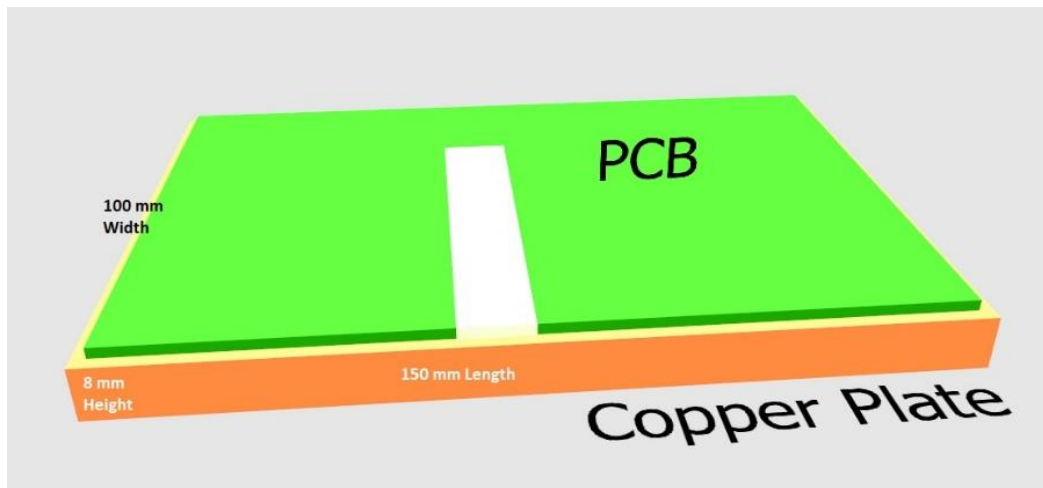
Figure-5: Mounting of RF amplifier PCB on copper plate
