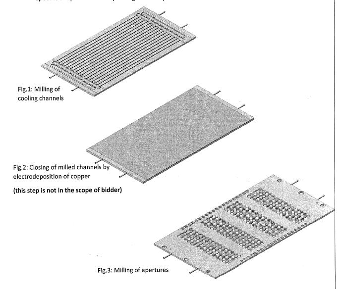
While the electrodeposition will be taken care by The Purchaser, we are looking for a competent machining company to perform the milling of the channels and drilling of the
