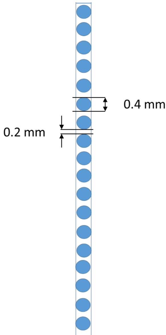
Vertical array of 18 optical fibers, with gap of 0.2 mm between each fibers
